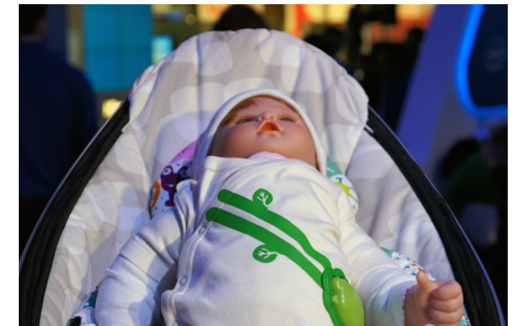
This smart data-collecting onesie for babies monitors heart activity and basic functions. It also activates other baby-gadgets according to the signals detected in the child.
