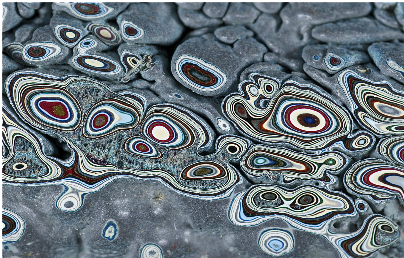
A section cut of Fordite, a paint sediment collected from the Ford factories of Detroit. Photo: Flickr/Agatehill
