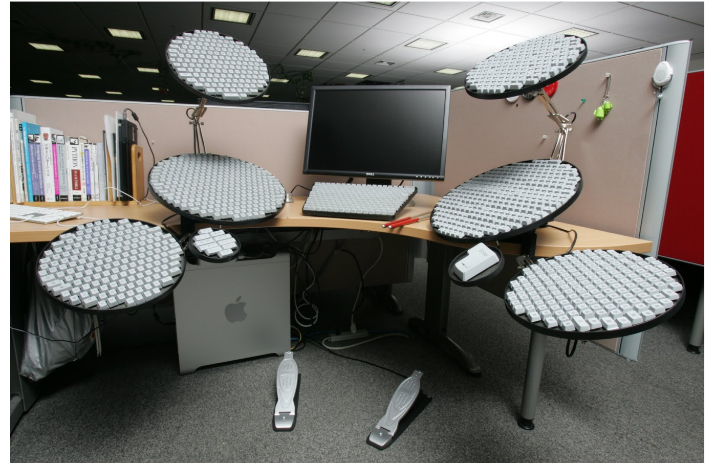
A tongue-in-cheek prototype of a Chinese computer keyboard, the first to feature one key per character instead of the multiple hidden commands required to type Chinese on QWERTY and Wubi keyboards.
