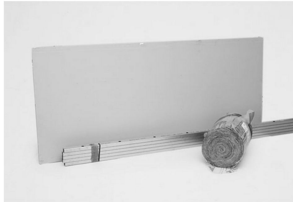
2 drywall panels (2.5m x 1.2m); roll of mineral wool insulation (16m x 60cm); 5 aluminum rails (4m x 3.5cm)— Purchased for €50.
